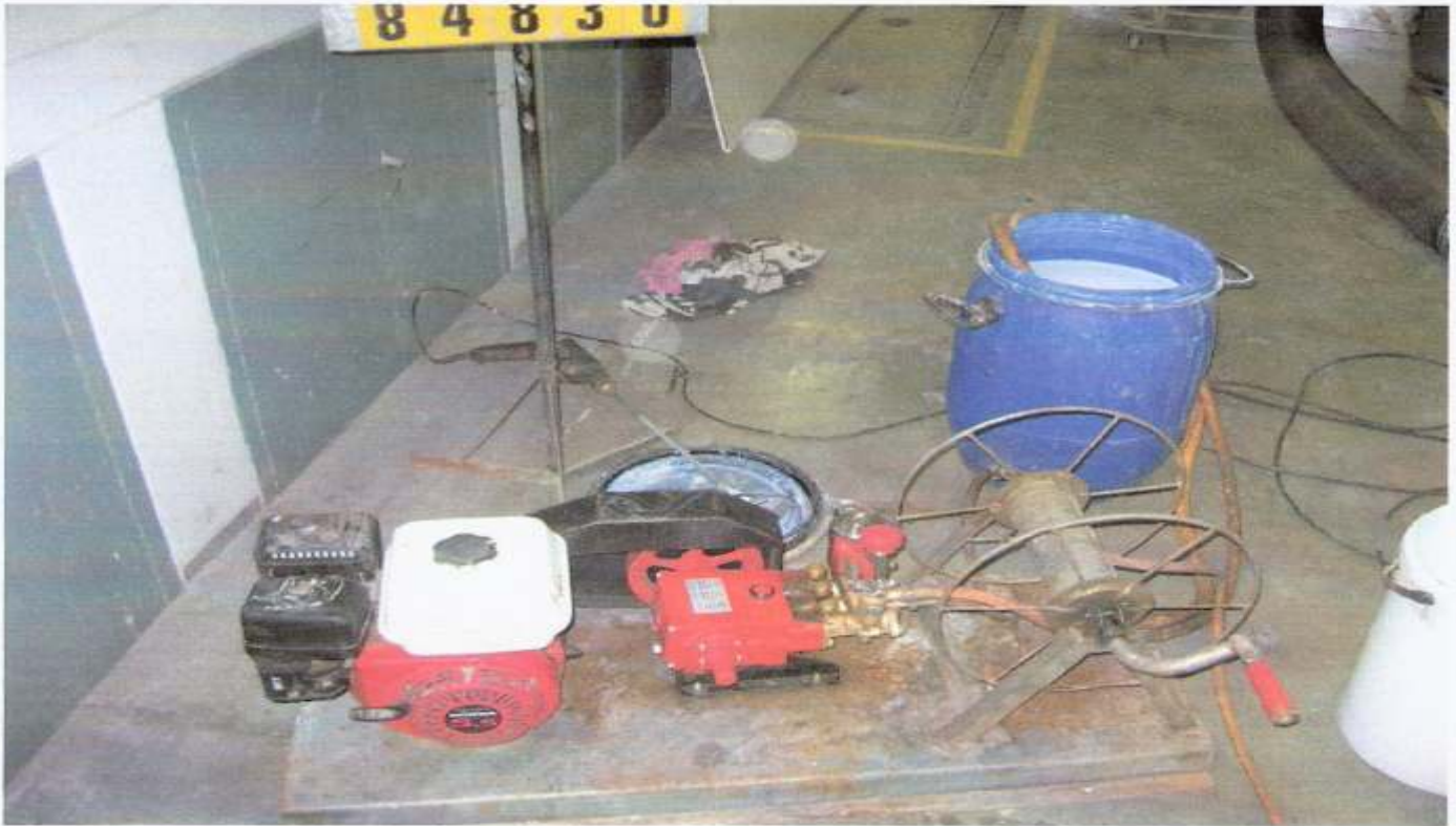
Photo 3 – Spraying equipment and Blues Pro in blue drum
