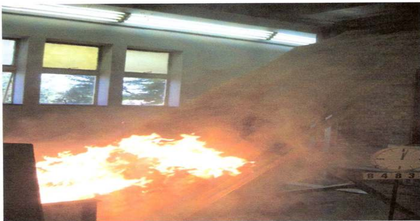
Photo 5 – Flame was ignited: 0 min
