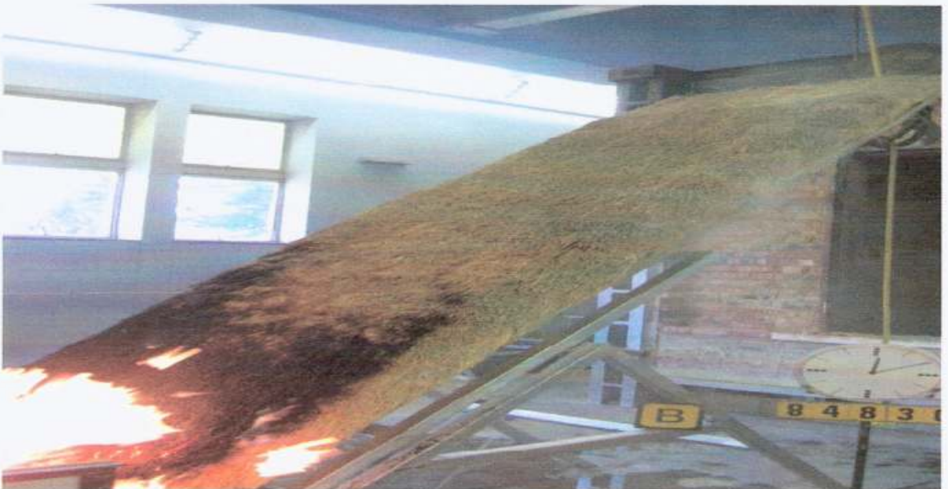
Photo 8 – Panel No 2 : On Completion of 10 min Flame Application
