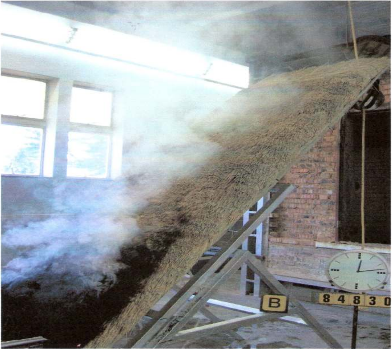
Photo 9 – Panel No 2 : 13 min No Flaming was observed on thatch panel
