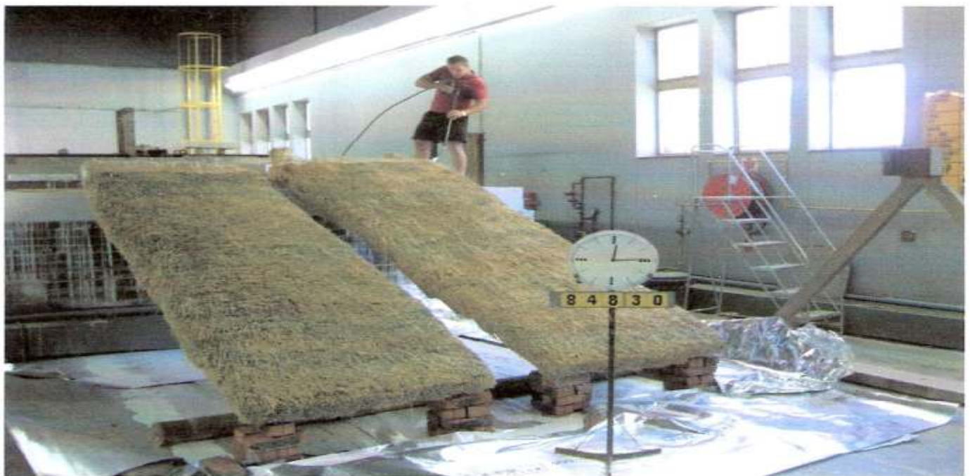
Photo 2 – Panel during spraying with Blus Pro FR 100
