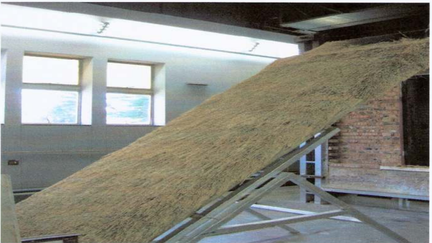
Photo 4 – Panel at onset of test
